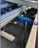
To protect the container itself from being stolen by lifting it off the chassis, an additional alarm system is installed. A motion detector fixed on the chassis framework registers any weight difference, with or without the container. When the container is lifted, a signal is immediately sent to the alarm system in the vehicle cab GPS/GSM.
