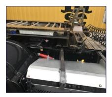
a sensor is installed. It connects the trailer with the driver's cabin through the saddle plate. The alarm is activated when an unauthorized decoupling occurs and sends an alarm to the vehicle cab and the AMC.
