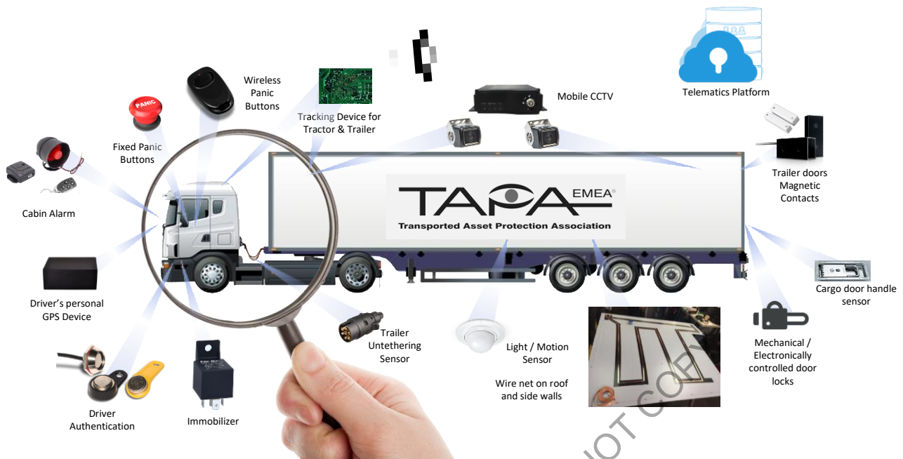
(Example of a telematics security system for a tractor and a trailer)
