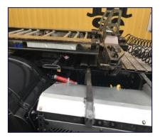
To detect and deter the chassis being stolen, a lock with a sensor is installed. It connects the trailer with the driver's cabin through the saddle plate. The alarm is activated when an unauthorized decoupling occurs and sends an alarm to the vehicle cab and the AMC.
