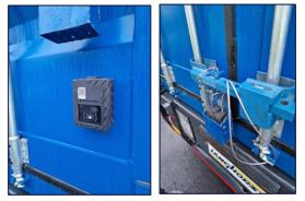
locks) to the GPS device. Therefore, if an attacker were to cut the cable or attempt to damage it or open the doors unauthorized, the GPS device would send an alarm or tamper alert to the agreedupon or system-stored locations (traffic planning department, driver, monitoring center, etc.).
