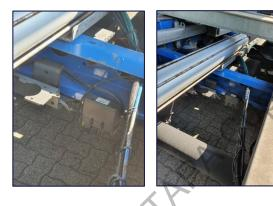
To protect the container itself from being stolen by lifting it off the chassis, an additional alarm system is installed. A motion detector fixed on the chassis framework registers any weight difference, with or without the container. When the container is lifted, a signal is immediately sent to the alarm system in the vehicle cab GPS/GSM.
