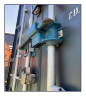
For further security, a special highsecurity Door Bar lock is installed. The features of this Lock are: The claws are forked and must be placed over the 2-door bar distance holders. The connecting bar, between these claws, is constructed of material that is resistant to drilling and flexing. Beam
